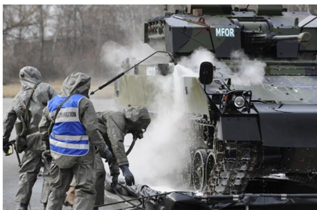
Decontamination of an armoured vehicle
